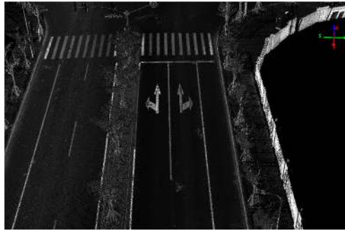
Figure 3. An example of the reflected intensity image of a laser scanner.
