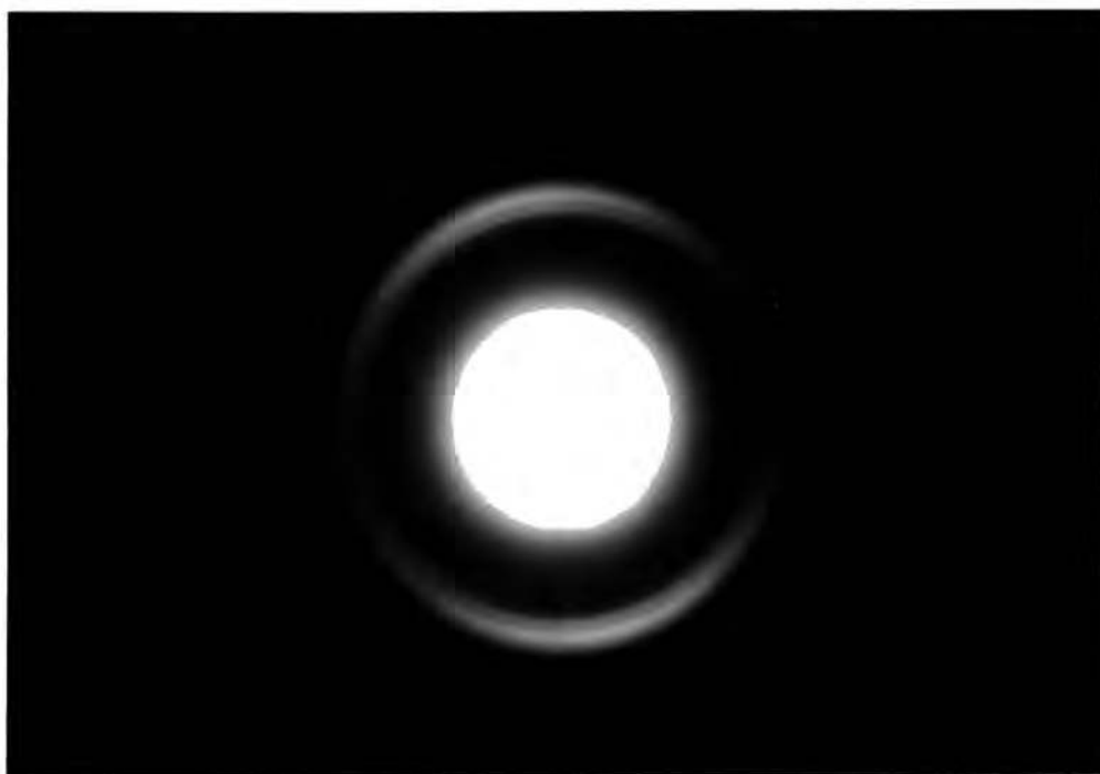
Figure 7.7 80kV TED pattern of an 11-layer LB film of amidonitrostilbene deposited on alumina.
