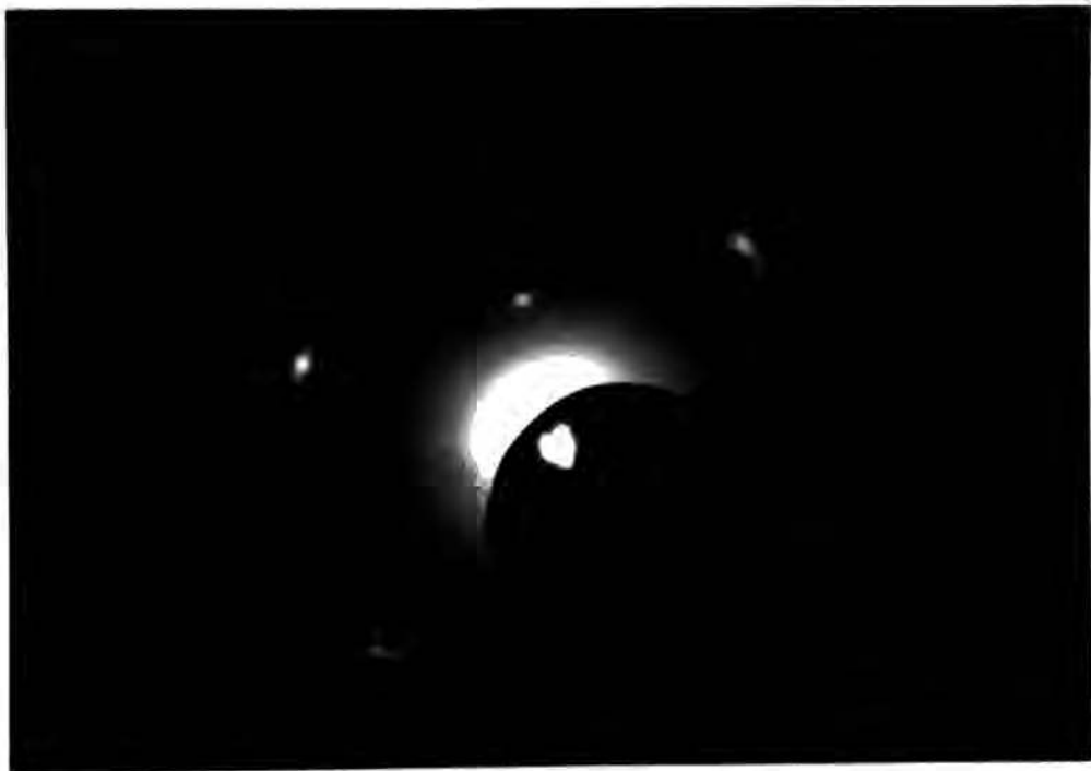
Figure 7.2a 100kV TED pattern of a 25-layer LB film of C4 anthracene deposited on alumina.
