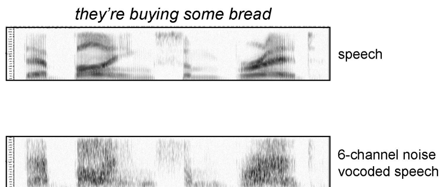
Fig. 1 Speech spectrograms of normal speech (top panel) and the same phrase as 6-channel noise-vocoded speech. Frequency is along the y-axis and time is along the x-axis. The amplitude at a particular frequency and time is represented by the intensity of shading.
