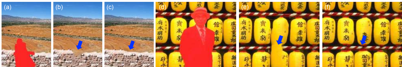
Figure 9. We compare the Gaussian-domain search (b) and (e) and our upsampled Gaussian-domain search (c) and (f). We set parameters the same for both methods and the patch size is 9 \times 9 for (b) and (c) and 5 \times 5 for (e) and (f). Under the same patch size, (c) and (f) captures global structures, while (b) and (e) misses the image structure.
