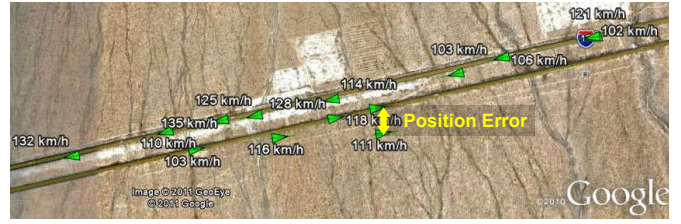
Fig. 5. GMTI result of the I15 data take as Google Earth overlay. The automatically detected road vehicles are depicted as colored triangles on their estimated geographical positions.
