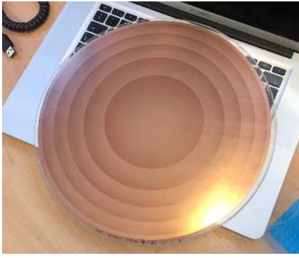
Figure 2. The completed 300mm metal mesh Fresnel lens.
