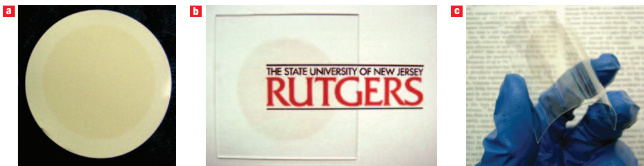
Figure 1 Thin films of solution-processed GO. a–c , Photographs of GO thin films on filtration membrane ( a ), glass ( b ) and plastic ( c ) substrates.
