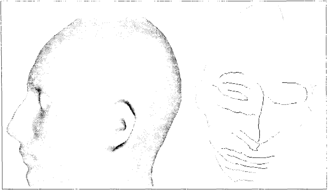
Figure 13: a. Left: Right profile of Carl with the 280 \times 160 grid. Note that the total amount of computing time needed is less than for the brute force method. b. Right: Crest lines are drawn on Carl's face after iteration fifteen, with our original method that measures local extrema of k_1^2 + k_2^2 on the surface (section 3).
