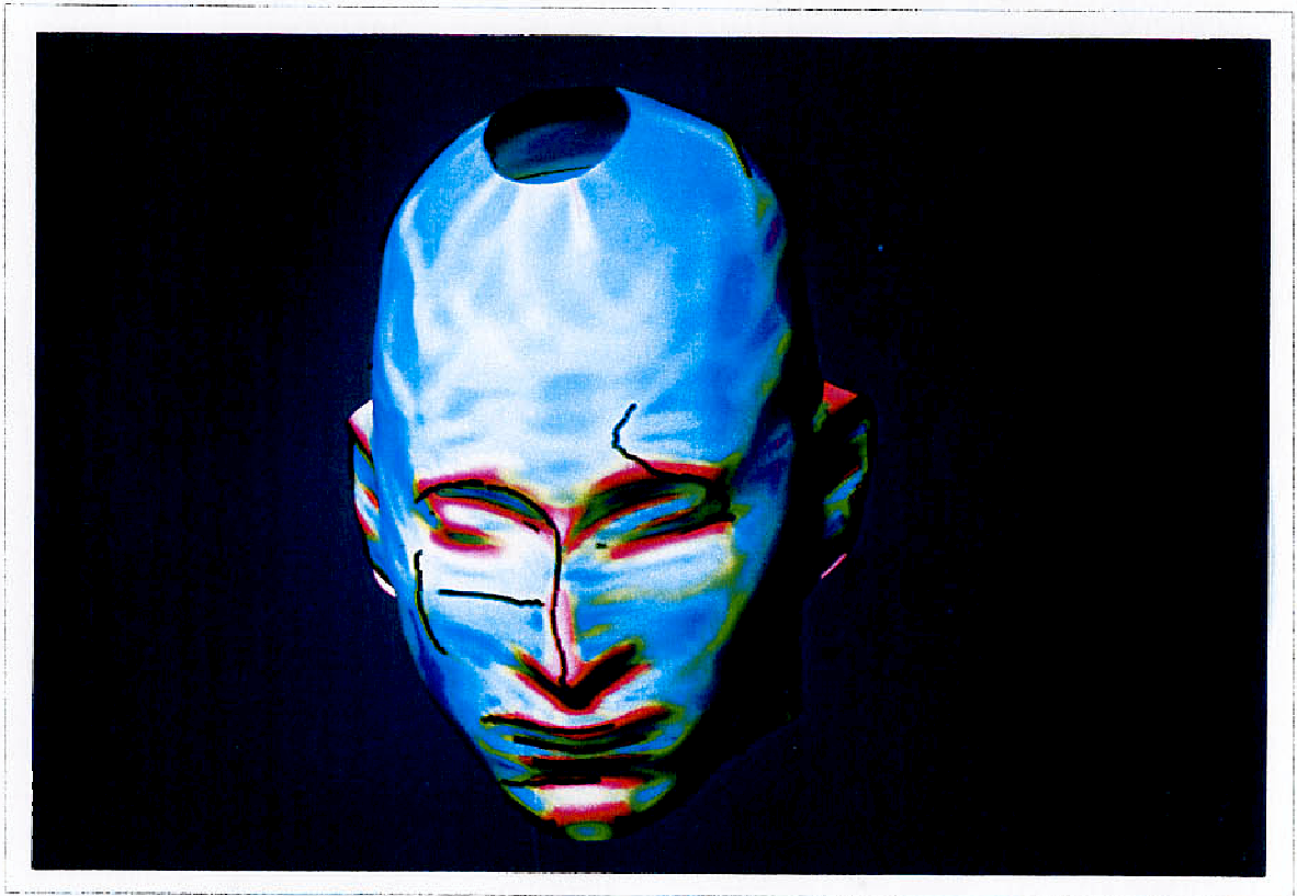
Figure 19: Rendered version of Carl with the AVS software. Crest lines are superimposed in black. (From lowest to highest curvature) blue, green, yellow, red color.
