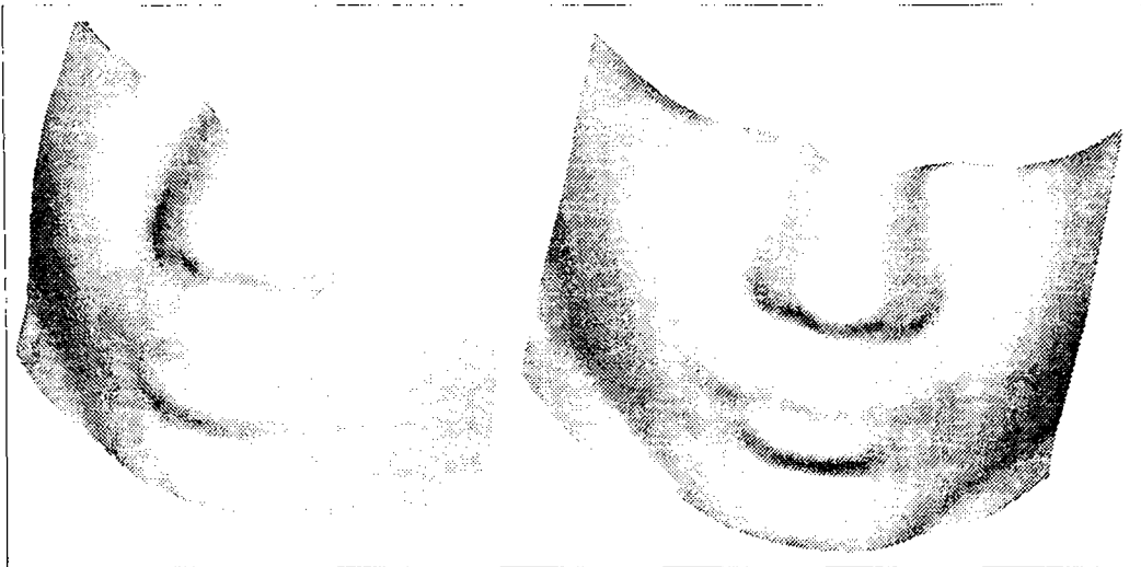
Figure 8: a. Left: Eighth iteration. The segmentation is almost complete. b. Right: Fifteenth iteration. The spline surface is stationary. Note that the spline could not fill up the lack of data at the tip of the nose.
