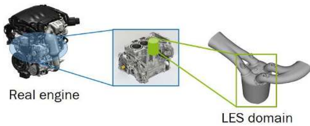
Figure 1. Presentation of the real engine configuration and the LES computation domain.
