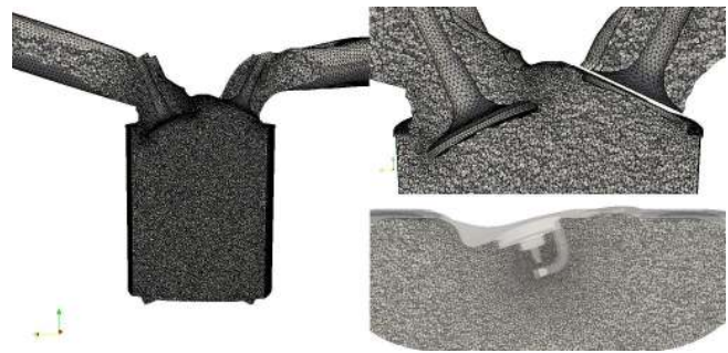
Figure 2. Presentation of meshes used during intake valve opening (left and top right) and at the spark plug during ignition (bottom right).
