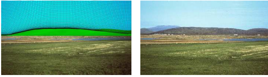
Figure 44. Left: The vertical meshing applied over the Askervein hill. The foreground has been taken from a photograph. Right: Photograph taken from an upstream location of the Askervein hill.
