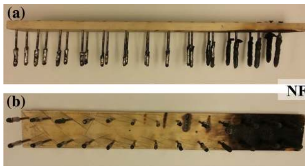
Fig. 21—Pictures of one of the nail boards used for the measurements at the commercial steel caster (a) front view and (b) bottom view.
