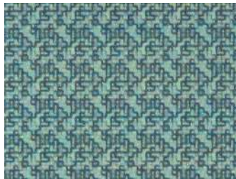
Fig. 2. Optical microscope image of a segment of the CGH disperser (Courtesy of D. W. Wilson and P. D. Maker, Jet Propulsion Laboratory).
