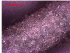
FIGURE 4. Micrograph of a monolithic slender element of the prototype showing granularity of printed Polyamide.
