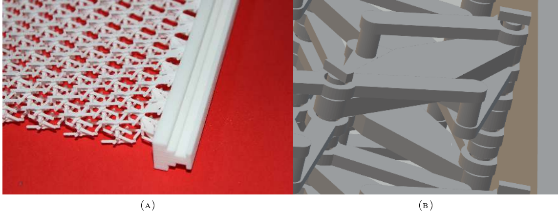
FIGURE 9. Realization of boundary conditions listed in Tab. 1. Manufactured specimen (A) and zoomed view of its CAD design (B).
