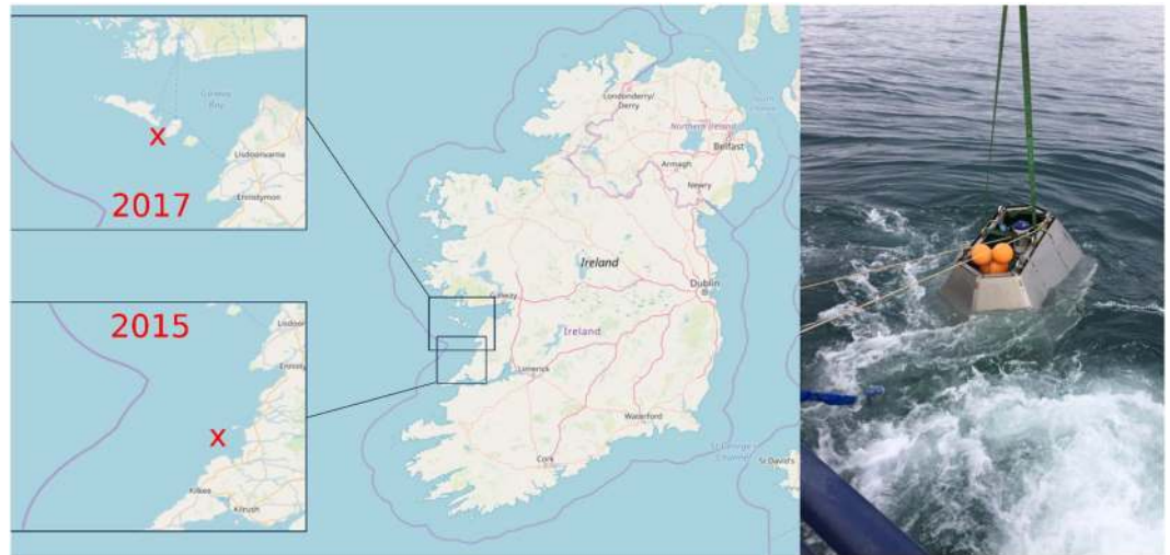
Figure 1. (Left) Map of Ireland: ADCP location off the Aran Islands in 2017 (upper Inset) and off Killard Point in 2015 (lower Inset). (Right) ADCP deployment with (blue-capped) instruments in a protective frame. The map was generated from data via OpenStreetMap and its contributors. Photo by F. Dias.
