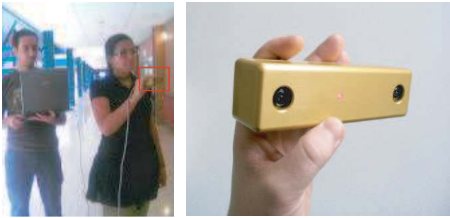
Fig. 1. Stereo vision system used to acquire the image sequences. Picture on the left shows the experimental setup during the data acquisition for the indoor experiment.
