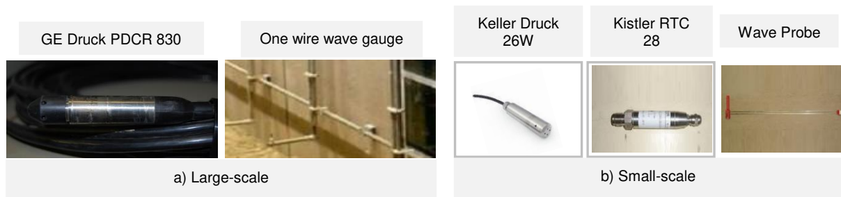
Figure 2. Large-scale (a) and Small-scale (b) instrumentations for measuring pressure and wave elevation.
