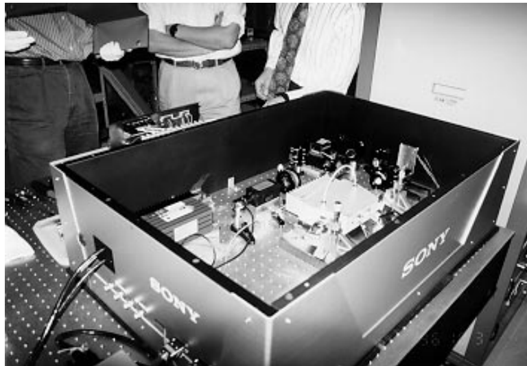
Figure 5: 10 W injection locked Nd:YAG laser system developed by Sony Corporation.
