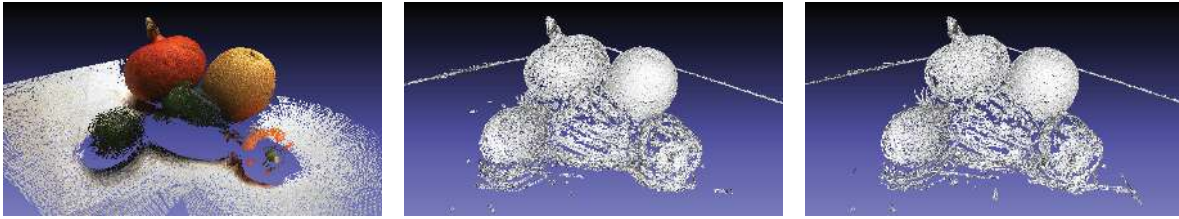
Fig. 11 An example of the effect of lighting variation. Left: our colored structured light reconstruction. Middle: the reconstruction of Fur [12] with full lighting. Right: the reconstruction of Fur [12] with varying lighting direction. The effect of varying the light seems negligible.
