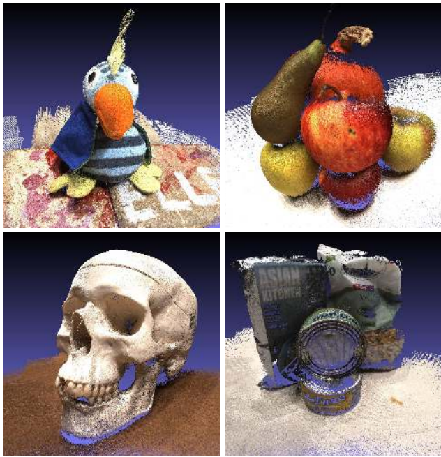
Fig. 1 Subset of point clouds in our reference data set. The images show point reconstructions of scenes with variability in geometry, reflectance, and texture. These images are grouped in our analysis into categories like groceries and vegetables.
