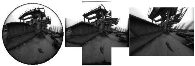
Fig. 2. Camera Models : The same image, warped to fit the three projection models considered in this paper. Both the Unified model and the piecewise rectified model can cover the full 185^\circ field-of-view. For the pinhole model, the image was cropped to a horizontal field of view of 120^\circ , which still causes significant stretching of the image around the border.
