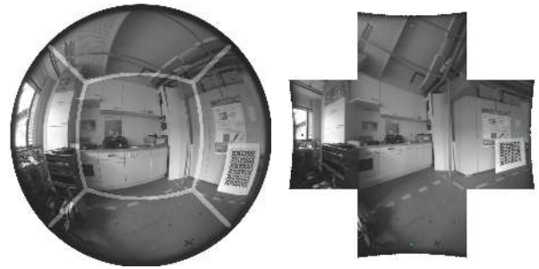
Fig. 8. Piecewise rectification: Example of fisheye camera rectification. The borders are still significantly distorted compared to the original image, as it is clearly visible on the checker-board, which leads to interpolation artifacts or blur.
