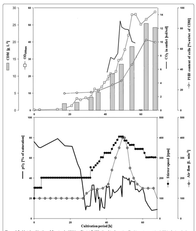
**Figure 1 Fed-batch cultivation of** *R. eutropha* **H16 in a Biostat D-650 stirred tank reactor.** The bioreactor contained 400 L of mineral salt medium with sodium gluconate as carbon source. A 20 L preculture was grown in the same medium. Cells were grown for 68 h at 30°C and harvested by continuous centrifugation. Due to technical problems, the concentration of carbon dioxide leaving the bioreactor could only be measured between the 40th and 58th hour.
