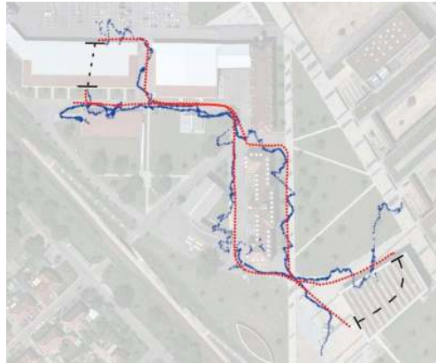
Fig. 7. Comparison between GPS measurements (blue crosses) and global poses from the localization in the aerial image (red circles). Dashed lines indicate transitions through buildings, where GPS and aerial images are unavailable.
