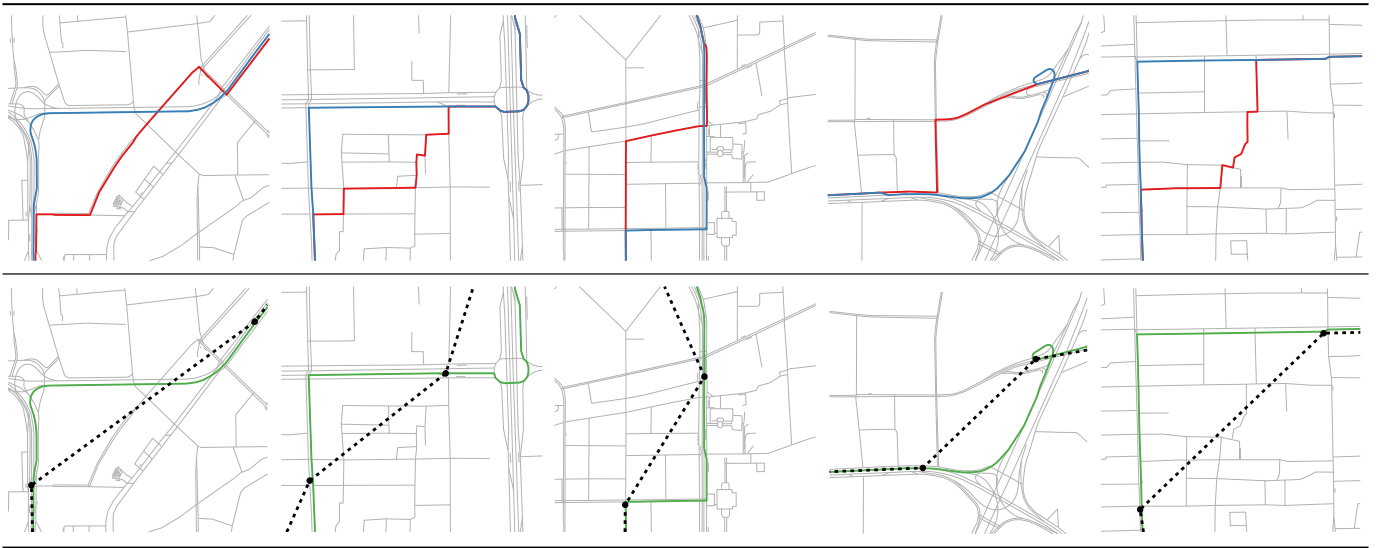
Figure 8: We show the difference between the map matching results of SMM (red) and data-driven map matching (blue) at intersections and curved roads. The bottom row displays the GPS sample points (black) and the manually matched path (green). In most cases SMM prefers "cutting the corner" while data-driven map matching tends to follow larger, popular roads, though the distance travelled along the two paths are very similar. This behavior conforms with the general observation that drivers prefer to stay on the same, faster route for as long as possible.
