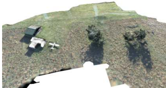
Fig. 1 A dense 3D mesh of rural farmland computed from sequential poses of visual SLAM from the air.
