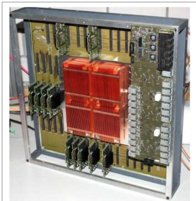
FIGURE 8 | Photograph of a BrainScaleS wafer module with part of the communication boards removed to show the main PCB. The wafer is located beneath the copper heat sink visible in the center.
