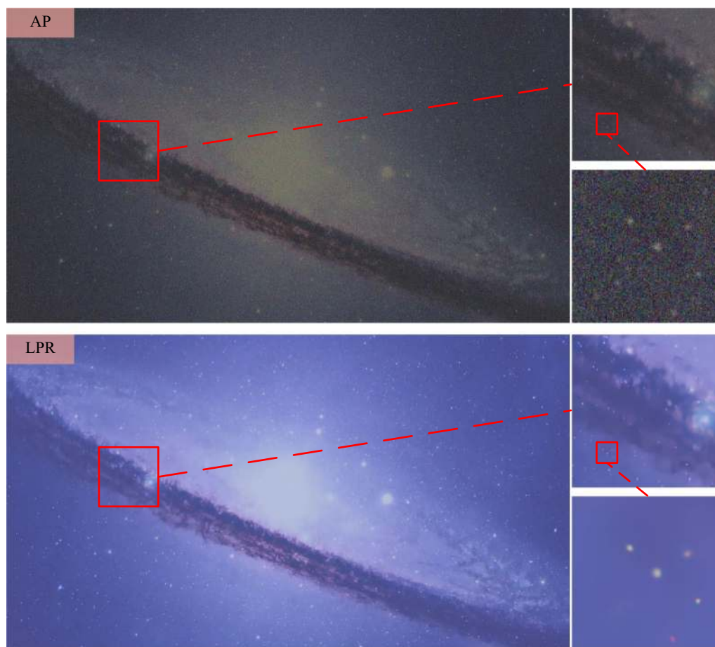
Fig. 6 The first demonstration of ultra-large-scale phase retrieval at the 8K level ( 7680 \times 4320 \times 3 pixels). The imaging modality is CDP with 5 modulations. At such a large scale, only the AP and the reported LPR techniques still work, while the other ones fail due to high computational complexity. The results validate that LPR significantly outperforms AP with effective noise removal and detail reservation
