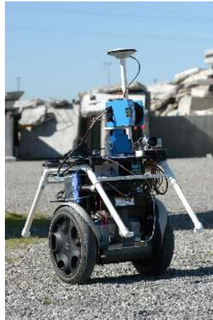
Fig. 1. The Segbot, a robot based on the Segway RMP platform and developed through the DARPA MARS program.
