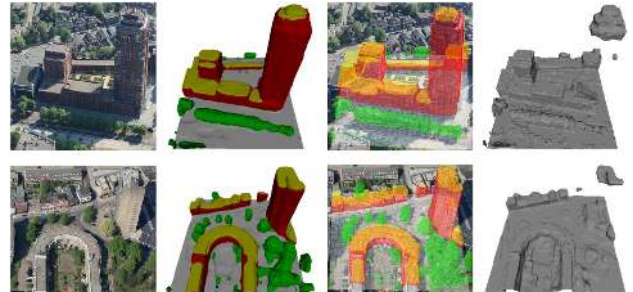
Figure 6: Left: Two images from the Enschede dataset. Middle left: Semantic 3D models (Scene 3 & 4). Middle right: Back-projected models overlaid on the images. Right: Pure volumetric 3D models [41]. Note errors such as deformed and fragmented buildings or flattened vegetation.
