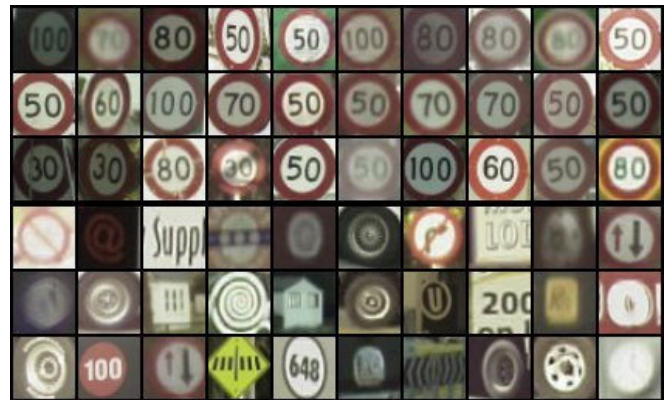
Fig. 1. New Zealand speed signs (top three rows) and challenging speed sign false positives (bottom three rows). The speed sign false positives shown here represent a tiny minority ( 5 \times 10^{-10} of windows scanned) of non speed signs remaining after a four stage classifier. Logos, wheels and other signs make up a large portion of difficult false positives. These challenging instances require more powerful features to further reduce the error rate of the classifier.
