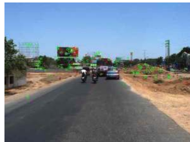
Fig. 4. Dynamic Object Detection: Matched features that were determined to be from moving objects are marked with red crosses, matched features that appeared to be stationary are marked with green circles
