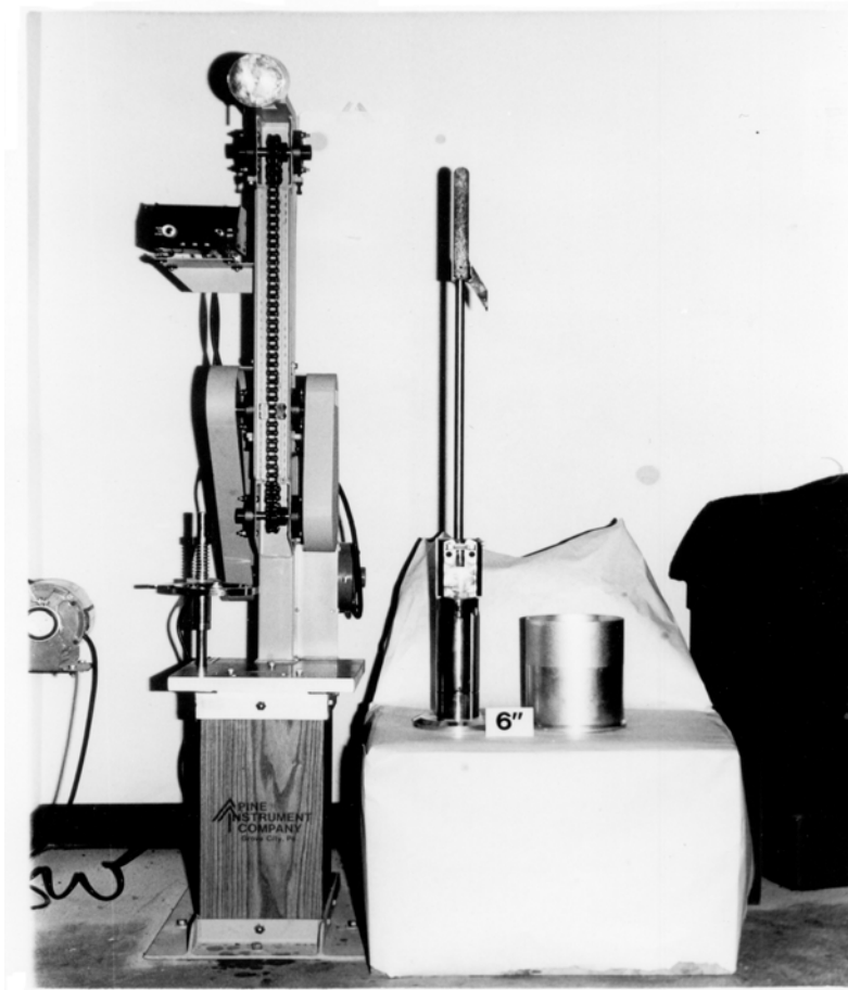
Figure 1. Compaction Assembly for 6-inch Marshall Specimens
