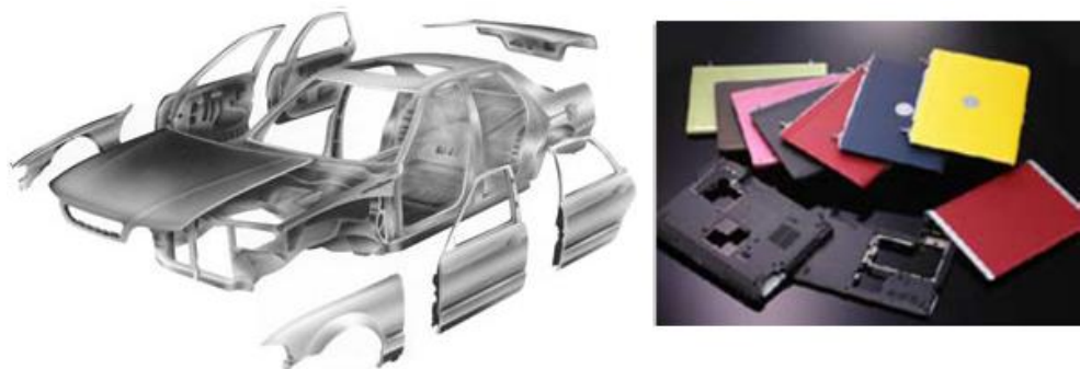
Figure 2.1. Examples of AHSS and lightweight sheet metal parts in automobile and consumer electronic applications [18, 19].
