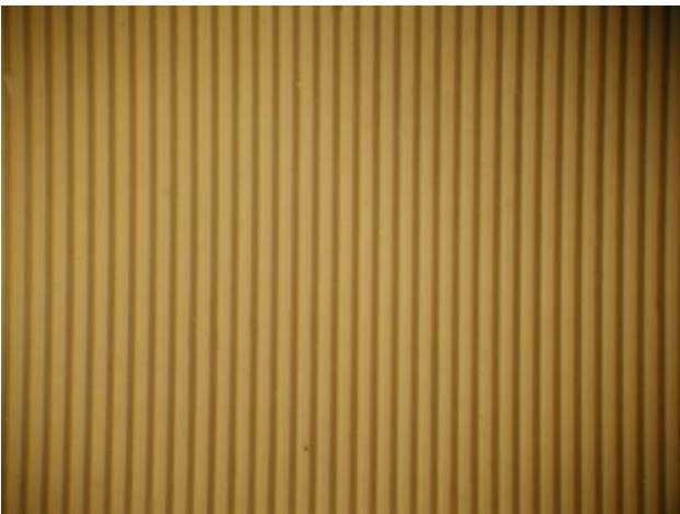
Figure 3: Stripes of YAG nanoparticles imprinted with Si gratings such as shown in Figures 1-2.
