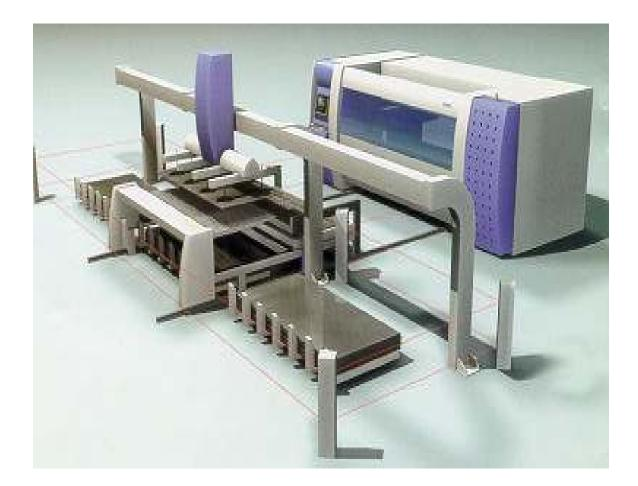
Figure 2.5: Laser-cutting machine with automated material handling
