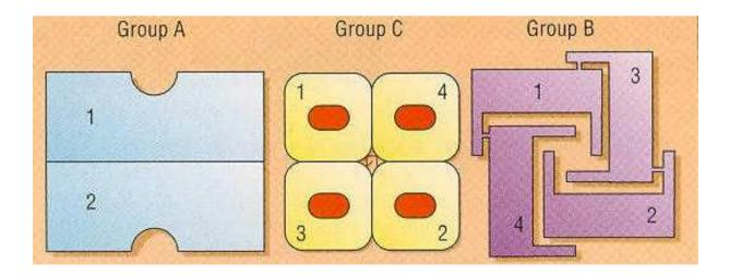
Figure 2.4: Illustration of commonline cutting and nesting
