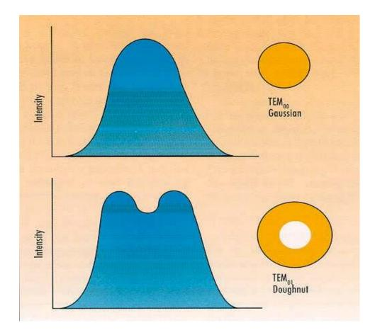
Figure 2.2: Types of laser beams
