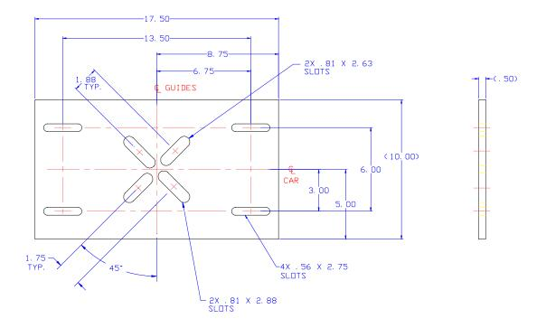
Fig.3.1: Sample of a new modular bracket.
