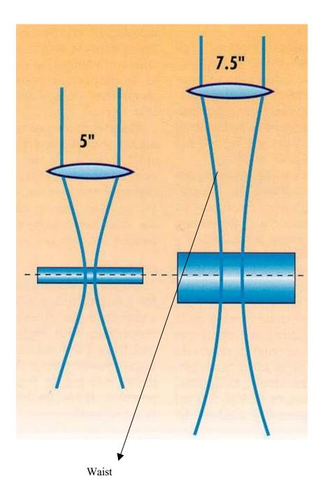
Figure 2.2: Illustration of 5" and 7.5" focal lengths
