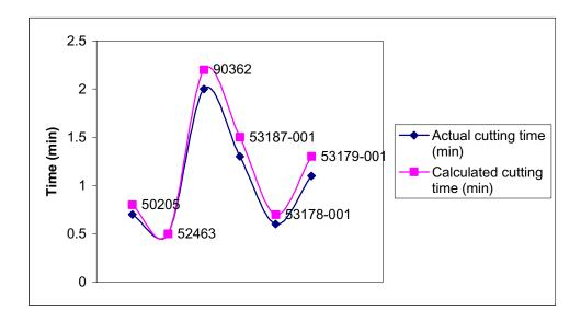
Figure 4.1: Graph showing the comparison between actual cutting time and calculated cutting time
