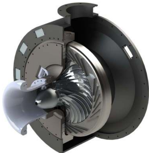
Fig. 1 Test compressor cross section
