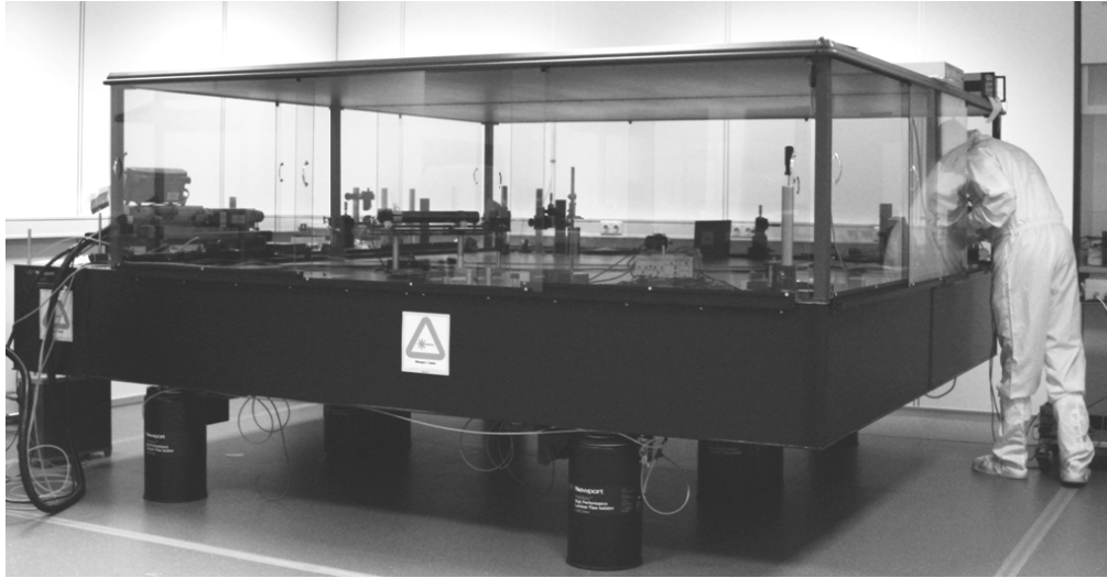
Figure 3. The Lloyd's Mirror interferometer on a vibration controlled table with air shield in the authors laboratory
