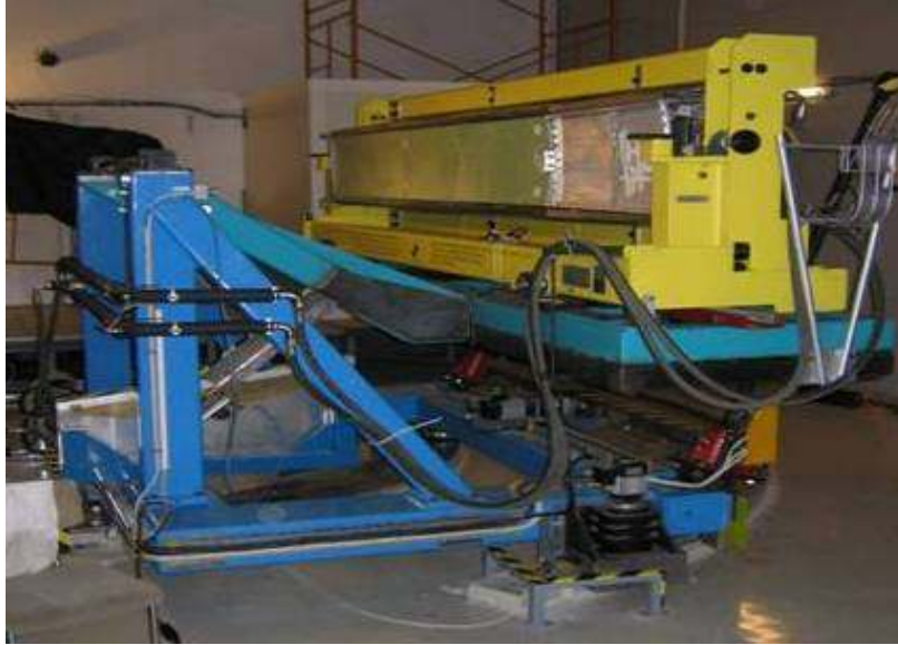
Figure 32. SM mounted on automated scanning table in CERN H4 electron test beam.
