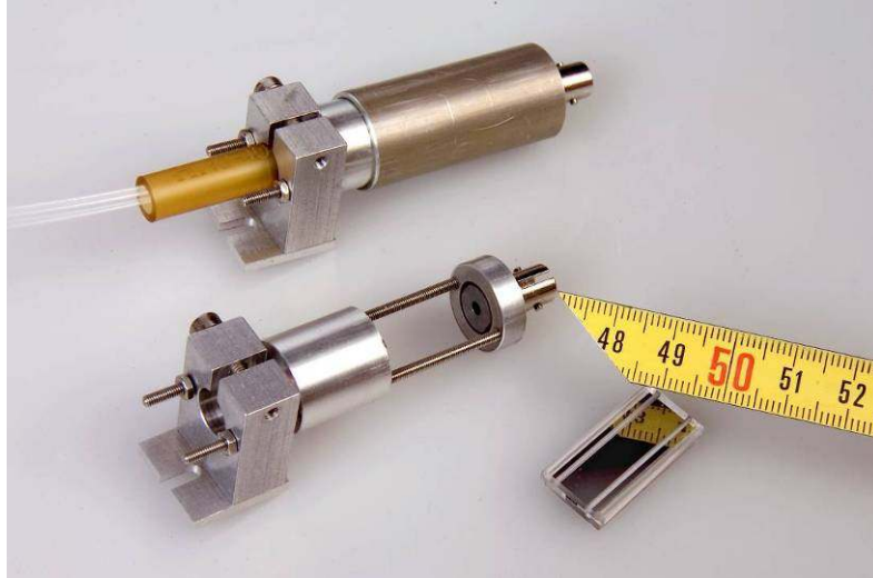
Figure 8. Secondary fan-out light splitter shown fully assembled above (light injection from right), and opened below with the 25 mm long light guide ( 1.7 \times 1.7 \text{ mm}^2 inner section) removed prior to bonding.
