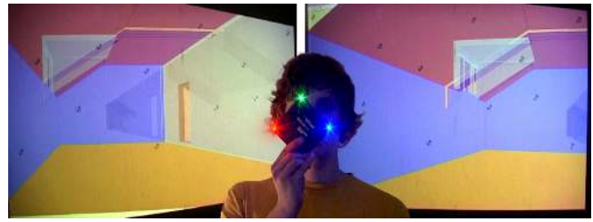
Figure 11: Two perspective views projected on the same surface. The viewer perspective is indicated with an active three-color LED marker.
