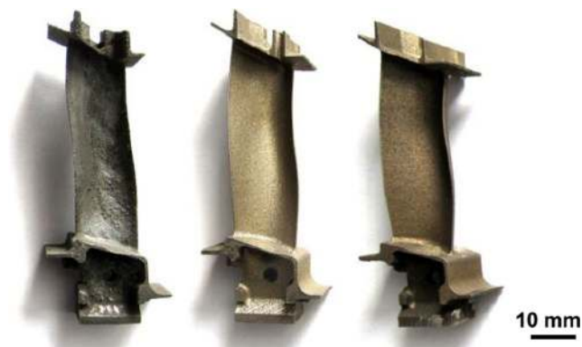
Fig. 12 Flat-, 45°, and upright-built turbine blades removed from the building plate and heat treated
