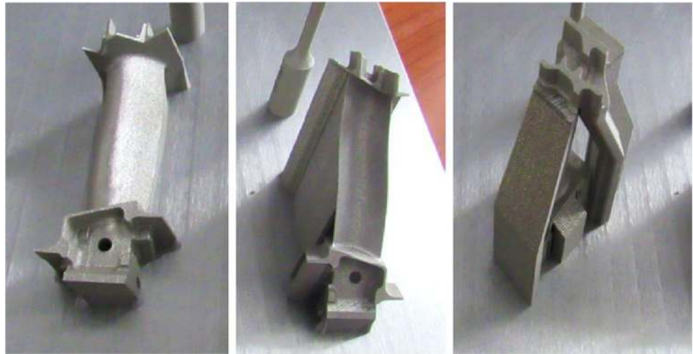
Fig. 11 Flat-, 45°, and upright-built turbine blades: as-built, with supporting structures on the building plate
