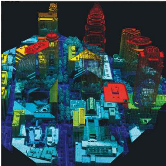
Fig. 28 Example of a 3-D urban data collection using a Geiger mode lidar. From Harris Corporation web page.
