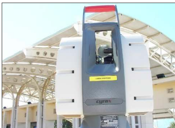
Fig.4: Laser scanner Leica HDS 3000
