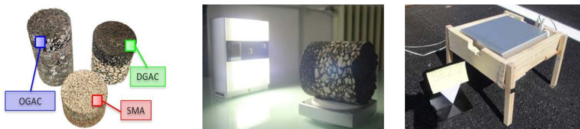
Figure 7. From left: road specimens, laboratory acquisition and on-site acquisition.
