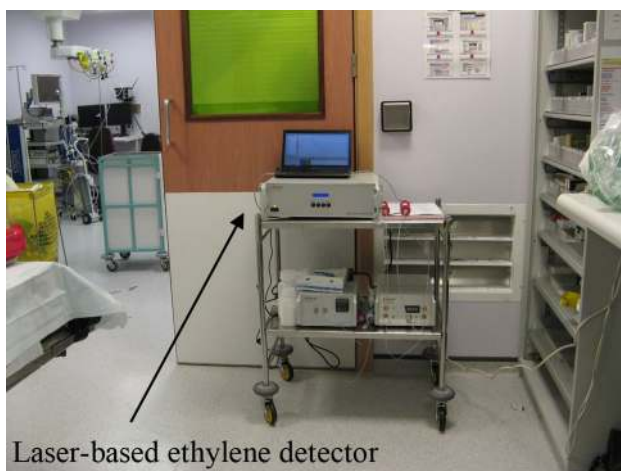
Fig. 5 Laser-based photoacoustic detector (ETD-300, Sensor Sense) in the cardiothoracic surgery department at Harefield hospital, UK (photo by S. Cristescu)
