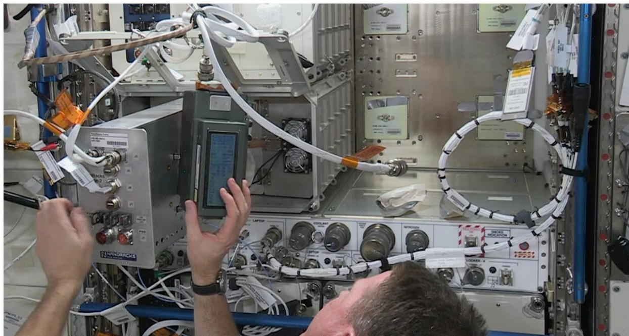
Figure 3. ISS crew member removing MGM from inside the locker where it monitored recirculated rack avionics air over a several month period, in support of the Fruit-Fly Lab that operated Jan 15-30, 2015.
