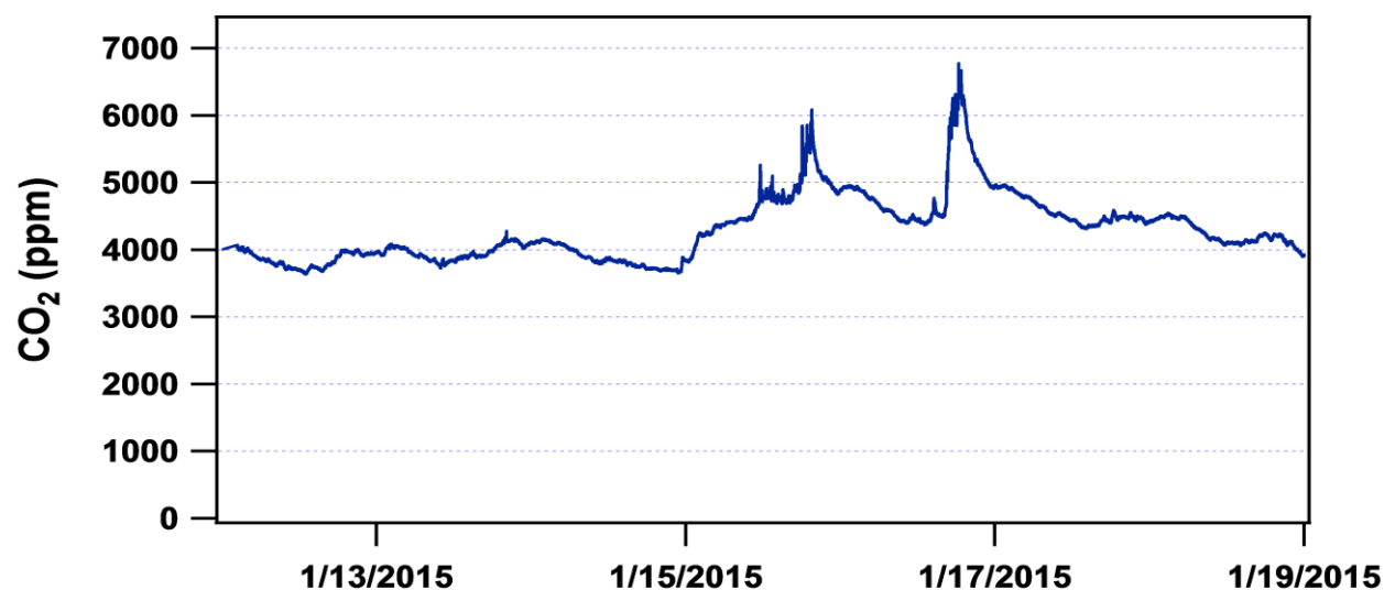
Figure 8. MGM again detected CO 2 increases as direct result of thruster firings from SPHERES Zero Robotics payload being operated in the JEM, the Dry Run on Jan 15, and the Competition on Jan 16, 2015.
