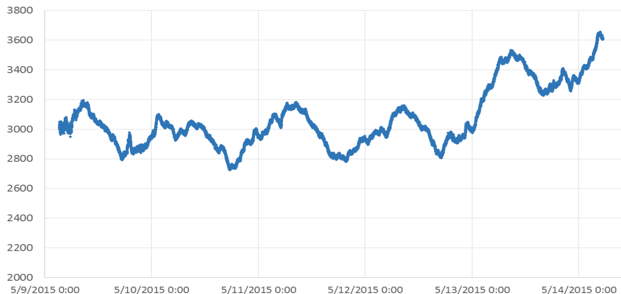
Figure 7. As of this writing, the most recently downlinked MGM CO 2 data in ppm, demonstrate ECLS control of CO 2 at or near the new operational target of 2.7 mm Hg (3600 ppm). Note the clear diurnal variations as well.
