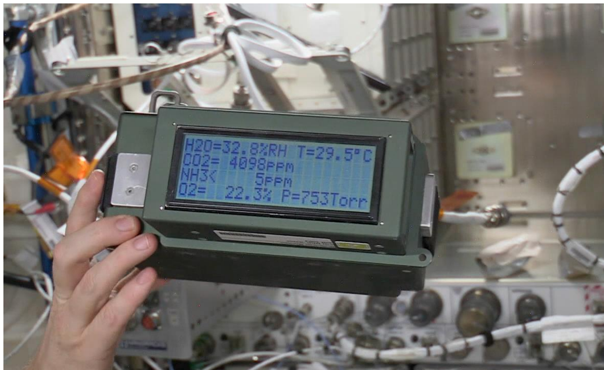
Figure 1. MGM being operated in battery powered mode in the JEM during Increment 42.
