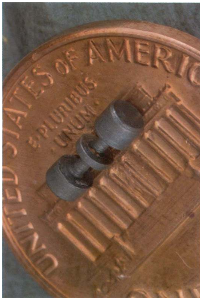
Fig. 2. The electrodes of a small rf trap, shown on a coin for scale.
