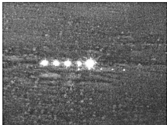
Fig. 1. Five laser beams incident on a dirt road, located 10 m in front of the vehicle. Image was captured with a SWIR camera.
