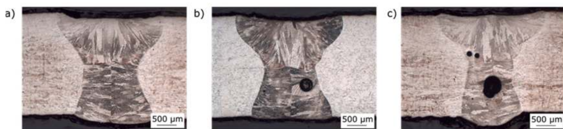
Figure 13. Cross sections of SLM-manufactured tubes of IN625 (overlap area): (a) IN625_WOHT_SLME, (b) IN625_HT_SLME, and (c) IN625_WOHT_SLME.
