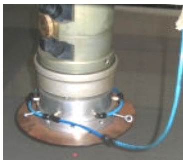
Fig. 2. Laser cutting head with cooling devices
