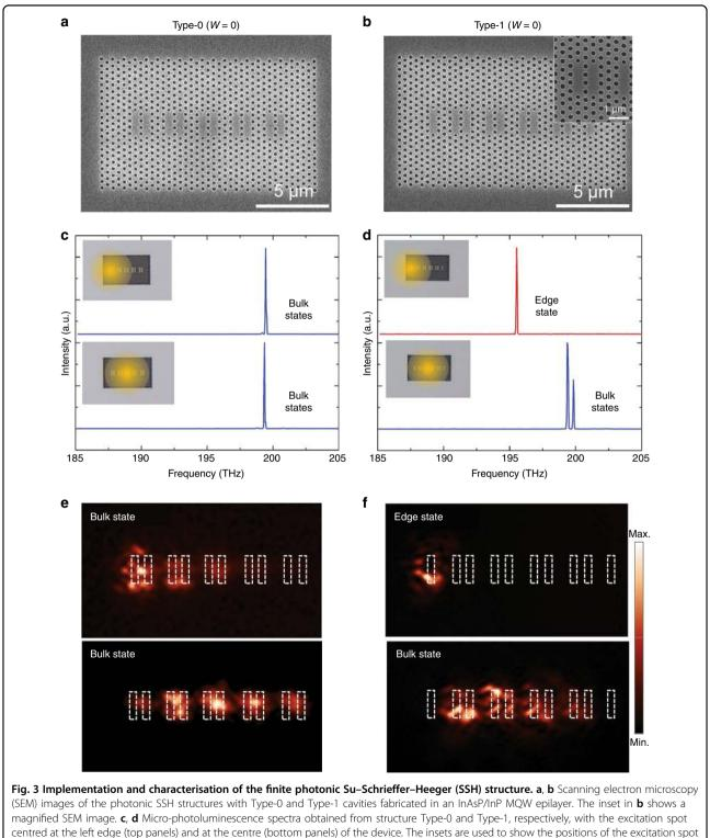
centred at the left edge (top panels) and at the centre (bottom panels) of the device. The insets are used to show the positions of the excitation spot (represented by the yellow-shaded circle) relative to the PhC nanocavity arrays. **e**, **f** Near-field scanning optical microscope (NSOM) images recorded for structure Type-0 and Type-1, respectively. The four NSOM images were measured at the corresponding peak emission wavelengths in **c**, **d**
