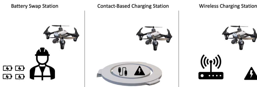
Figure 4. This figure illustrates the three types of battery replenishing stations for drones.
