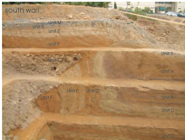
Figure 5. Photo of the south wall showing a 32° east-dipping main thrust and the fault scarp that was formed by the Chichi earthquake. The hanging-wall structure is a broadly open anticline, and the footwall is characterized by a syncline with the axial surface approximately parallel to the thrust.
