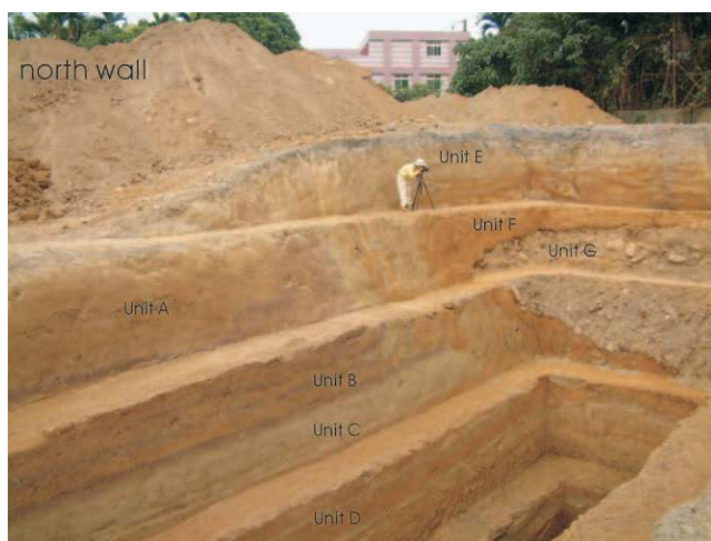
Figure 6. Photo of the north wall showing a tight anticline with a steeply inclined (overturned) forelimb on the hanging wall.
